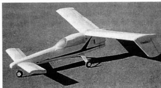
The Canada Goose Canard's tricycle landing gear. Propeller clearance on takeoffs and landings is critical for rear-engine canards.
