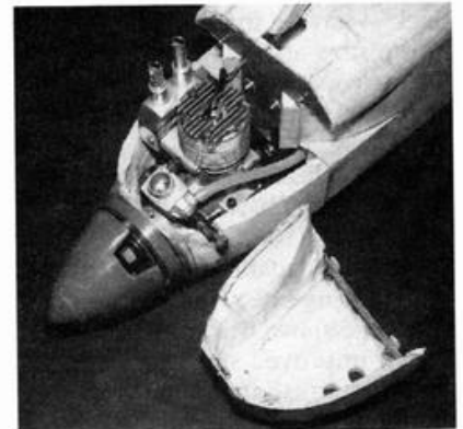
Photo D. This cowl detail shows that servicing the engine is easy.
