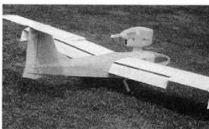
The Seagull III—an amphibious flying boat. Powered by an O.S. Max 46SF engine, it weighs 113 ounces and is an excellent performer. Its large slotted flaps are fully extended for landing.
