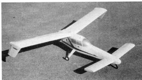
The Canada Goose is a canard that uses the low-drag techniques described in this chapter.
