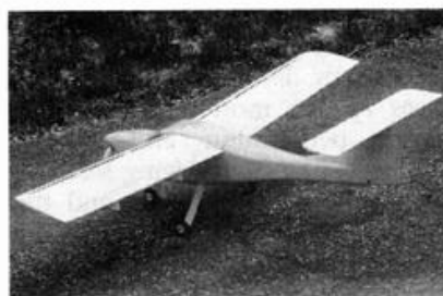
The Crow at rest. Note the wing's high-lift devices (HLDs).
